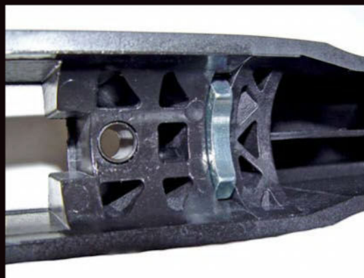
The Axis II's stock contains a metal lug that fits into a slot machined into the bottom of the rifle receiver.
