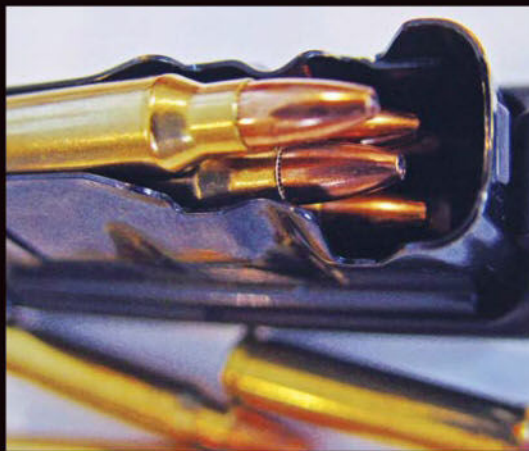
The removable magazine is designed to hold four cartridges.
