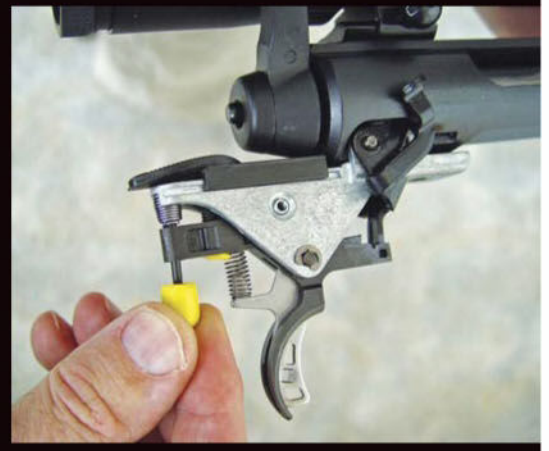
A small tool is included with each Axis rifle for adjusting the trigger pull.
